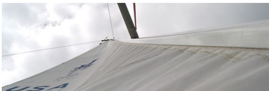
1”-3/4” of sag to leeward indicated proper lower shroud tension
