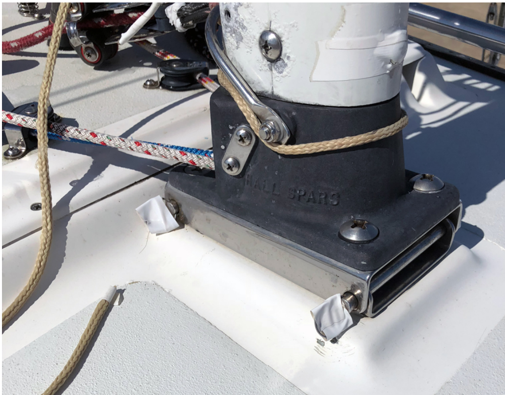
Two pins hold the J/22's mast in place.
